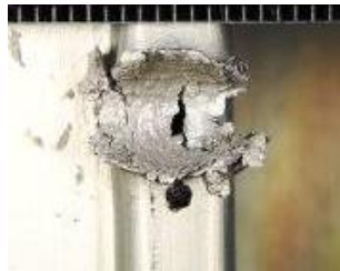
Phase VI Glove Vectran damage from simulated MMOD
