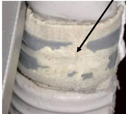
TurtleSkin® Patch after cycling on simulated MMOD
