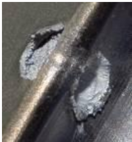
On orbit MMOD damage
