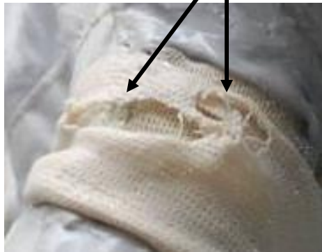
Phase VI Glove Vectran damage from simulated MMOD
